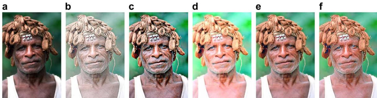
Fig. 1. Algorithm comparison: (a) original image taken from [15], (b) enhanced RGB channels, (c) MSR with color correction [15], (d) LDNE [20] [21], (e) RR [5] [6] [19], and (f) enhanced with the approach we propose.
